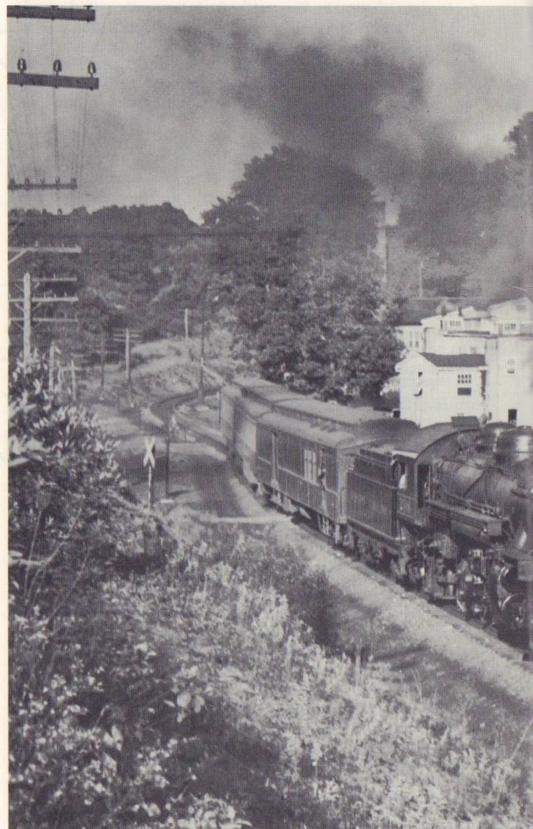
Fig. 7-13. Two immaculate Western Maryland three-car passenger trains stage a classic meet at Westminster, Md. To the dispatcher such a meet looks the same as a meet between a 100-car drag and a 17-car limited. For the single-track enthusiast, choice of era, locale, and railroad should be such as to favor stubby consists and thus permit a choice of meeting points in spite of the necessary brevity of the main line.
