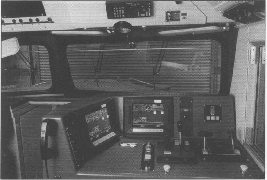
Fig. 4-11. General Electric Desk Top Console With Two PC Screens
