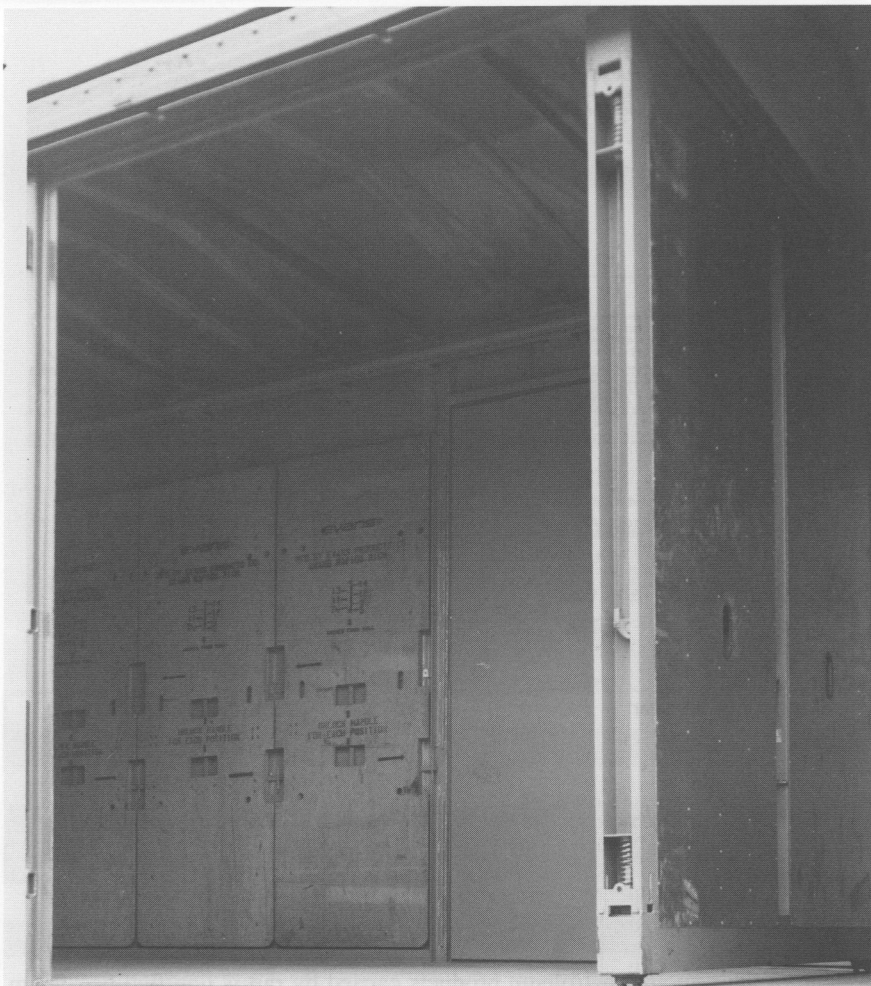
Fig. 9-16. Typical Load-Restraining Device Used in DF Car
