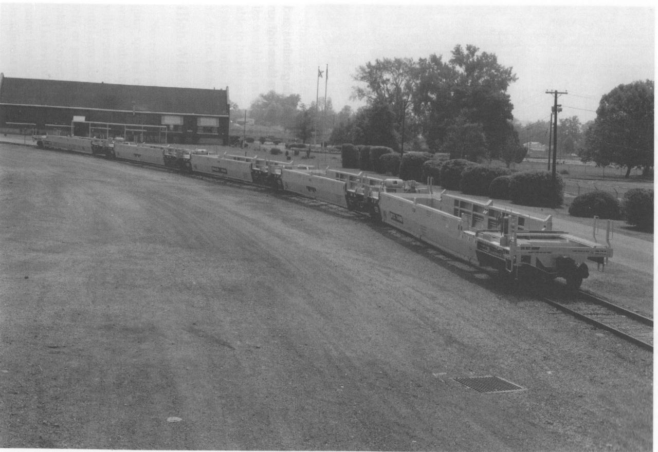
Fig. 15-6. Five-unit articulated 48' well car with 125-ton intermediate trucks, adaptable for double-stacked ISO marine (8' wide) or domestic (8'6") containers.
