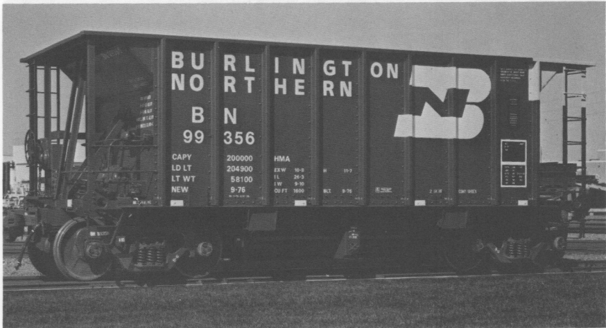
Fig. 9-4. HMA Ore Hopper Car
