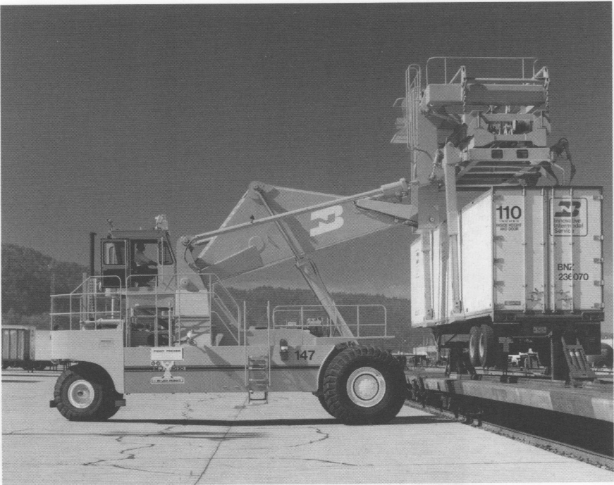
Fig. 15-7. Mobile side loader ("piggy-packer") capable of loading trailers and containers on single or double-stack rail cars, stacking containers three high on ground.
