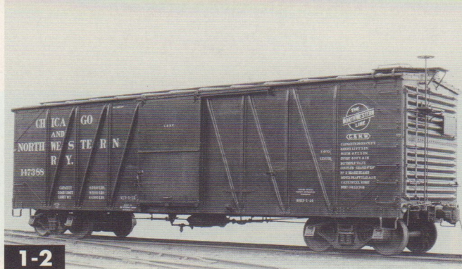
1-2 This single-sheathed USRA-variation boxcar was built in 1925. It has Murphy ends with a 7/8 pattern. The underbody brake gear is readily visible on these cars. David P. Morgan Library collection
