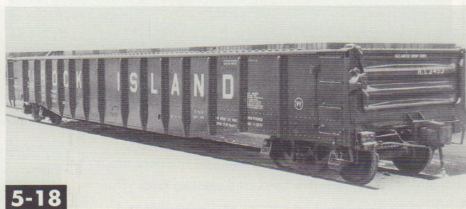
5-18 Among the most common mill gondolas of the late steam/early diesel eras was the drop-end, 53'-6", 70-ton car first built by Greenville. This Rock Island car was built by Pullman-Standard in 1957. Drop-end gons have lever-style brake handles. Rock Island
