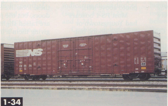
1-34 Gunderson built several excess-height 60-foot cars in the 1990s, including this Norfolk Southern car. Jeff Wilson
