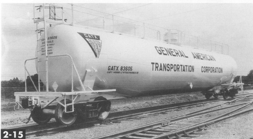
2-15 "Pregnant whales" such as this 70-ton car were popular in the 1960s. This 30,000-gallon General American car was designed for carrying LPG and anhydrous ammonia. Timken Roller Bearing Co.
