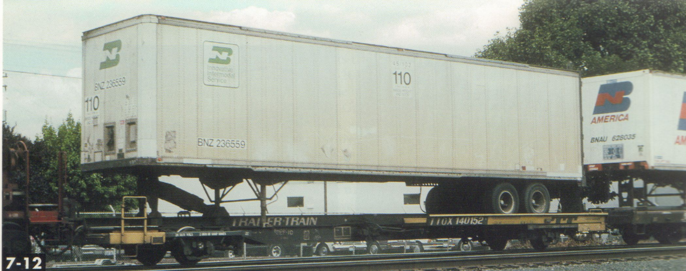
7-12 Front Runner cars are single-unit lightweight platforms with single axles at each end. This car was built by Paccar in 1984. Jeff Wilson
