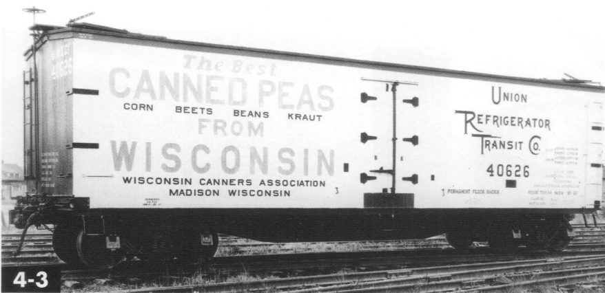
4-3 This 40-foot Union Refrigerator Transit RS car is typical of reefers built into the 1920s. It has a steel fishbelly underframe and wood body, including ends and sides. Hol Wagner collection
