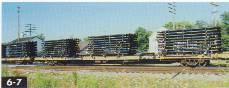
6-7 TTX has converted many former piggyback cars for other uses. One example is this car for hauling pipe, a Pullman-Standard car with S-shaped side channels. Jeff Wilson
