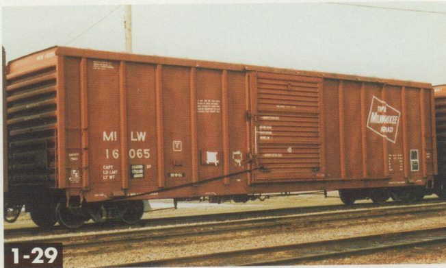
1-29 The Pullman-Standard 5,344 cubic-foot boxcar was a common 1970s car. It had a flat roof that wrapped around the tops of the sides and posts, and non-terminating ends with closely spaced corrugations. Jeff Wilson collection
