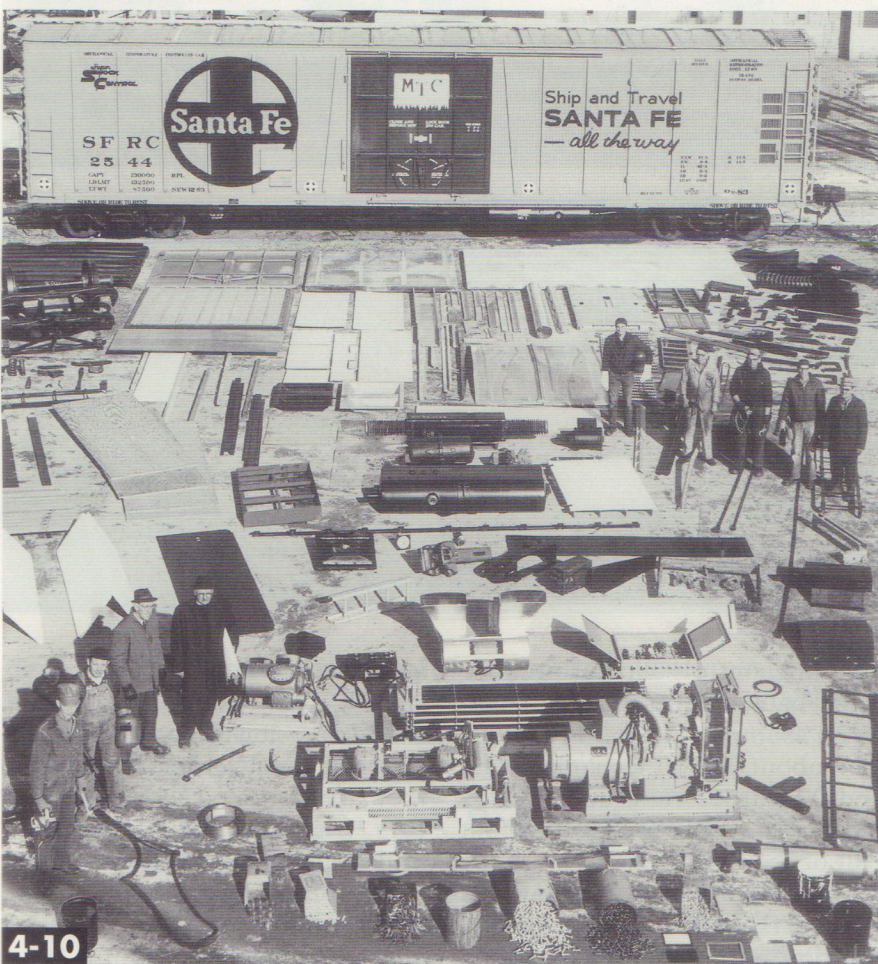
4-10 This Santa Fe publicity photo shows the parts that go into a mechanical reefer. The car, built in 1963, is 60 feet long with exterior posts, cushion underframe, and a nine-foot plug door. Santa Fe
