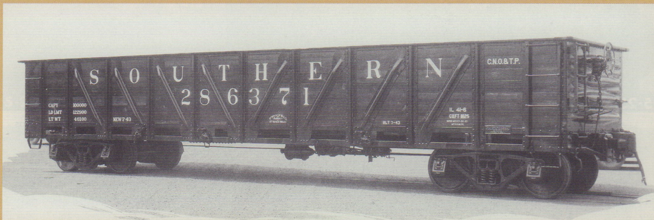
This war-emergency gondola has six drop doors and an inside length of 41'-6". It was built in July 1943. Mt. Vernon Car Manufacturing Co.
