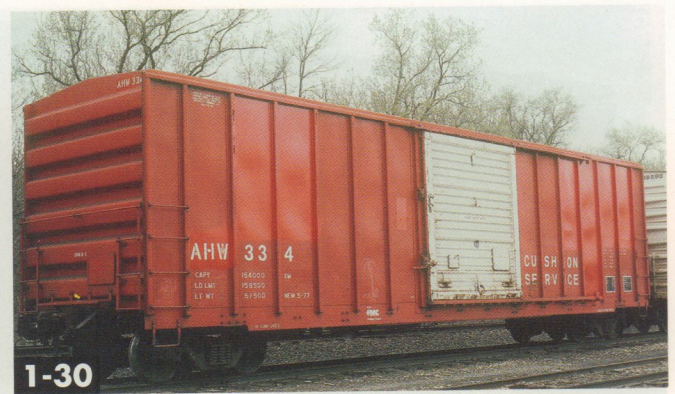
1-30 This FMC-built car has non-terminating ends, a peaked roof, and a different sill design than the ACF car in figure 26. Jim Hediger
