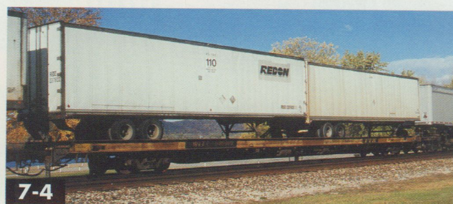
7-4 Bethlehem's channel-side cars were the most common 89-footers in Trailer Train's fleet. This car is carrying a full load of two 45-foot trailers. Jeff Wilson
