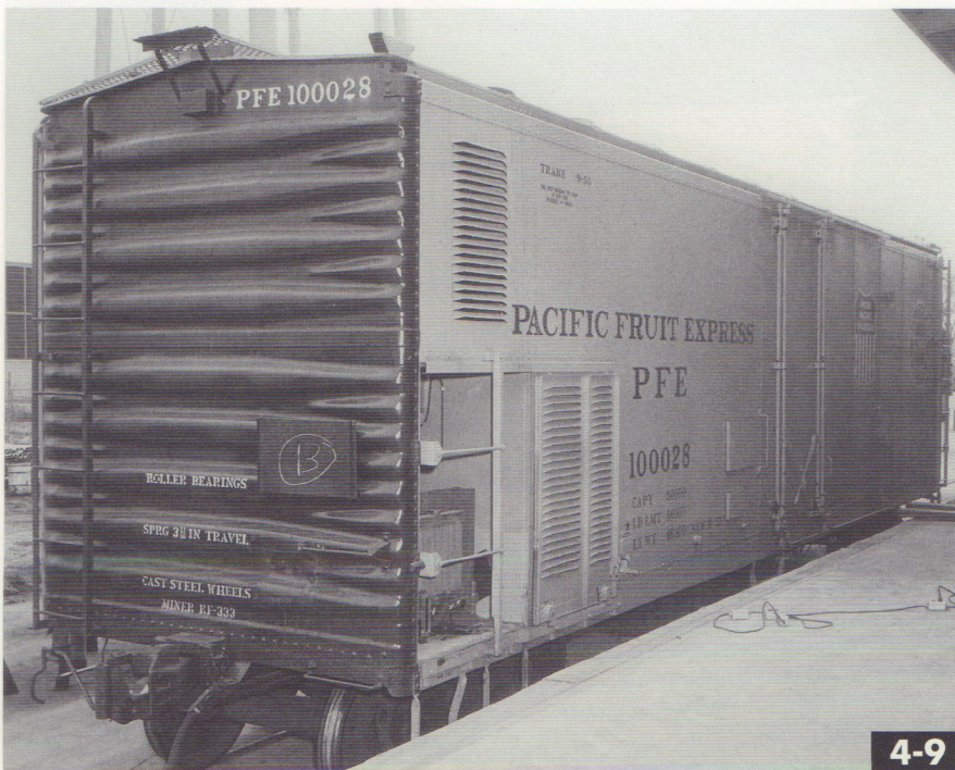
4-9 The refrigeration equipment in this 1958-built Pacific Fruit Express R-40-30 mechanical reefer is clearly visible in this photo. The 40-ton, 40-foot car has sliding plug doors. William Harwood
