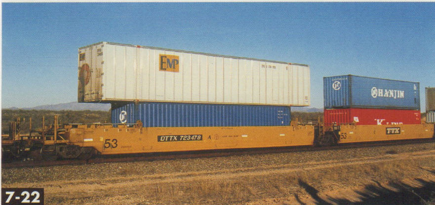
7-22 Gunderson's 53-foot cars resemble its earlier 48-foot cars, but with deeper sides. This is a three-unit articulated car. Jeff Wilson
