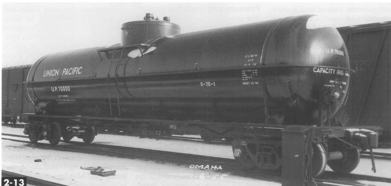
2-13 Tank car size began increasing in the 1950s. ACF built this welded 70-ton, 19,000-gallon ICC103W car in 1954 for Union Pacific. Union Pacific
