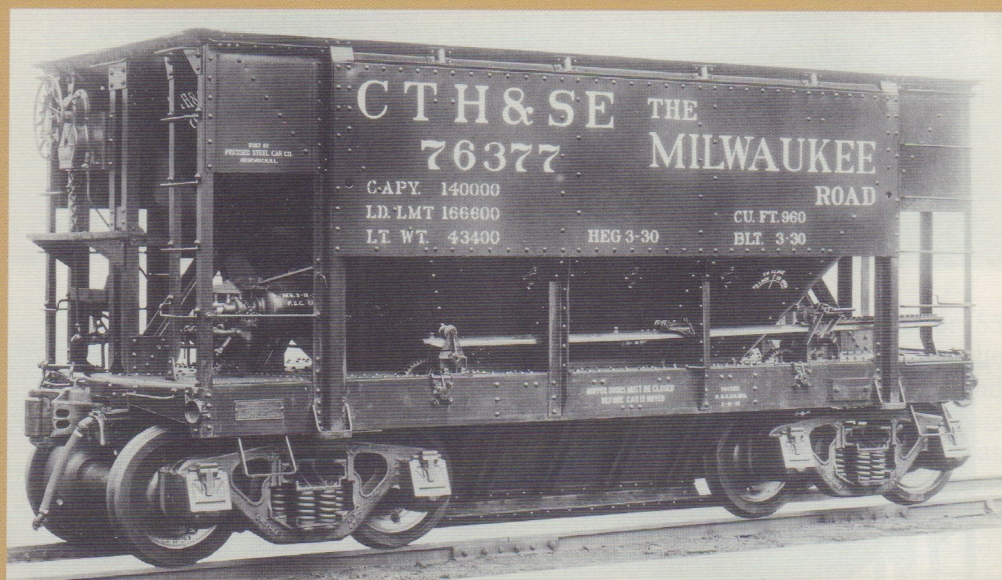
Ore cars are significantly smaller than standard hoppers because of the high density of iron ore. This 70-ton car was built in 1930. Pressed Steel Car Co.
