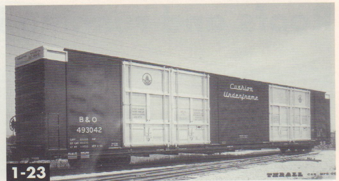
1-23 Thrall was second in 86-footer production. Note the recessed side sills on this four-door car built in 1966. Thrall
