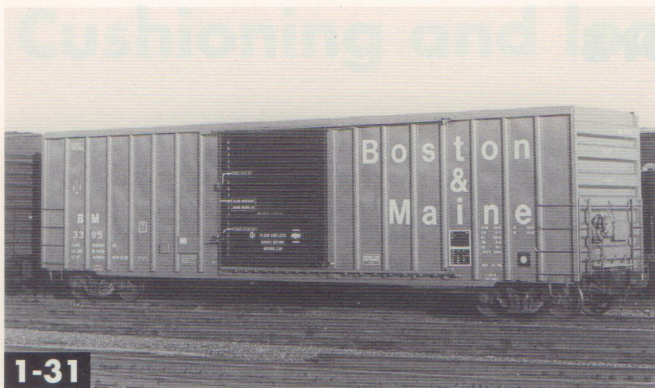
1-31 Pacific Car & Foundry built this Plate C car for Boston & Maine with a flat roof and non-terminating ends. The car has 14 posts per side. Tom Nelligan
