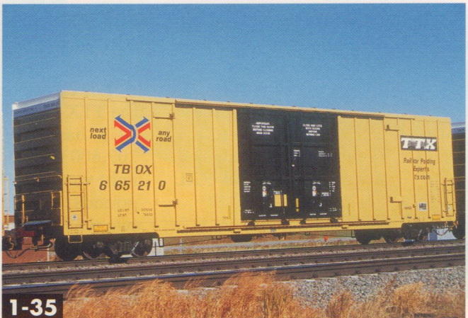
1-35 Among the newest cars on the rails in 2005 are TTX's TBOX cars, such as this one built by National Steel Car. They're primarily used to transport paper and paper products. Jeff Wilson
