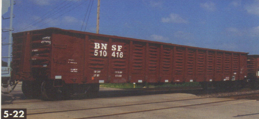
5-22 A popular 1980s variation was the use of horizontal corrugations for extra strength in the panels. This is a 100-ton Burlington Northern Santa Fe car. Bob Gallegos
