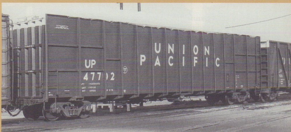
Modern wood-chip cars are excess height (note the white end panel) with an end door for dumping. Note the mesh screen covering the load.
