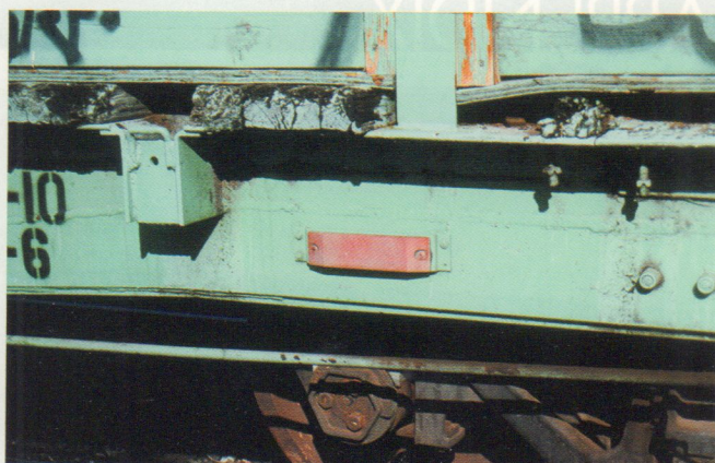
Automatic Equipment Identification (AEI) tags were required on cars as of 1994. These use passive radio signals to transmit data to railside scanners, avoiding the grime problem that plagued the earlier ACI system. You'll find tags on each car side, toward the right end of the car. Jeff Wilson photo
