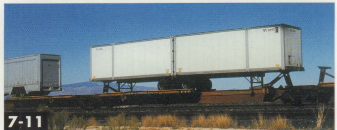
7-11 Platforms of Twin-28 spines can haul single long trailers or containers or a pair of back-to-back 28-foot trailers. Jeff Wilson
