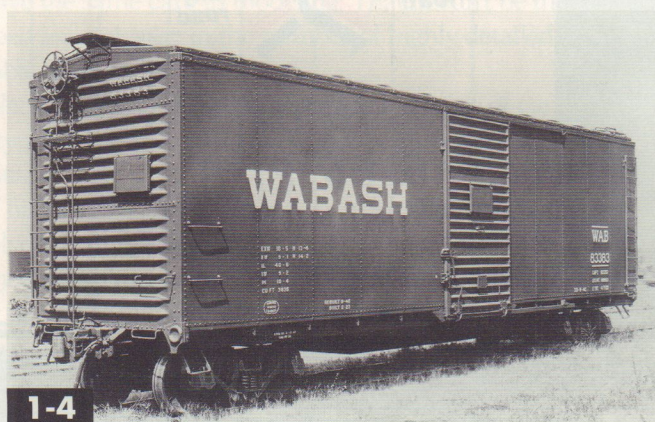
1-4 The original deep fishbelly underframe is still visible on this rebuilt USRA boxcar. The wood sides have been replaced with steel, the Murphy ends extended to make the car taller, and a new power hand-brake (Miner) has been added. David P. Morgan Library collection
