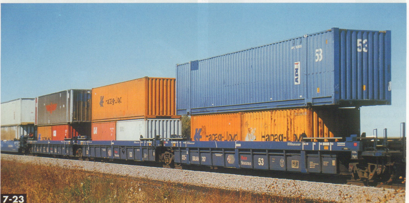
7-23 Thrall's 53-foot articulateds have the same characteristics as the company's earlier cars, with vertical exterior posts and squared-off ends. This is a three-unit car. Jeff Wilson
