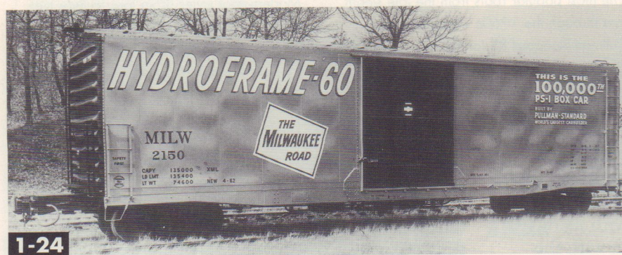
1-24 Pullman-Standard modified its PS-1 with a continuous-tapered sill in the early 1960s. This 50-foot car has the company's Hydroframe-60 cushioned draft gear and nine-foot-wide doors. Milwaukee Road
