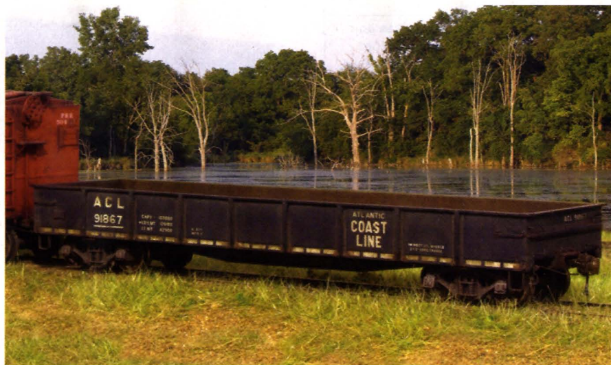
Fig. 3 Fish-belly center sills. Modeler Jim Six modified an Ertl HO scale 42-foot gondola with a fish-belly center sill to backdate the car to model a specific Atlantic Coast Line prototype. Jim Six photo
