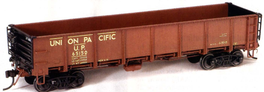
Fig. 7 General Service (GS) gondolas. Red Caboose makes this model of an AAR class GS gondola. Equipped with bottom doors, these cars carried loads as diverse as coal, crushed stone, beets, rails, pipe, and machinery.
