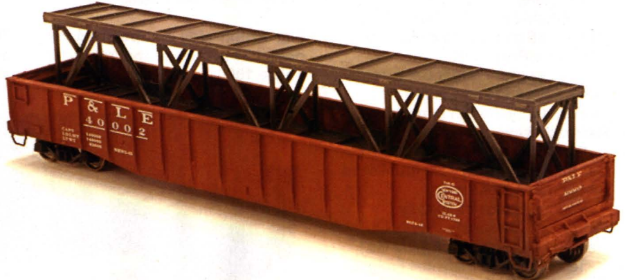
Fig. 6 Steel girder loads. Gondolas were often built to handle standard lengths of structural steel. A 50-foot deck girder span fits readily into a 52-foot gondola. Jerry Glow built this Proto 2000 kit replacing grab irons with ladders. The bridge span is from a Micro-Engineering kit. Tony Koester photo
