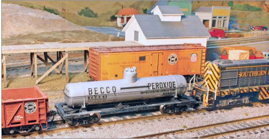
25. The completed peroxide tank car, with Champ decals for Buffalo Electro Chemical Company (Becco) applied. This is a Plastruct tank with K&S aluminum tubing for the dome, and a variety of detail parts used for the dome top.
