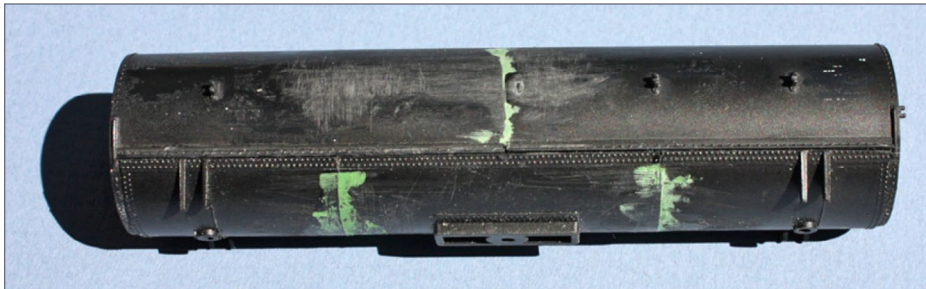
14. An Athearn insulated tank body, shortened to fit the InterMountain frame, and reassembled. Cuts in the top and bottom pieces are differently located (see text). Longitudinal rivets seen here are incorrect and were removed.
