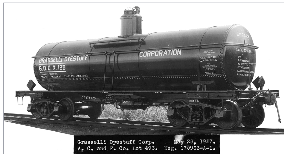
25. A typical acid tank car, Class ICC-103A, with its distinctive dome shape and appliances. The car was built in 1927 and has 50-ton trucks and 7045 gallons capacity, typical for cars carrying dense acids. (AC&F photo, courtesy Edward S. Kaminski)
