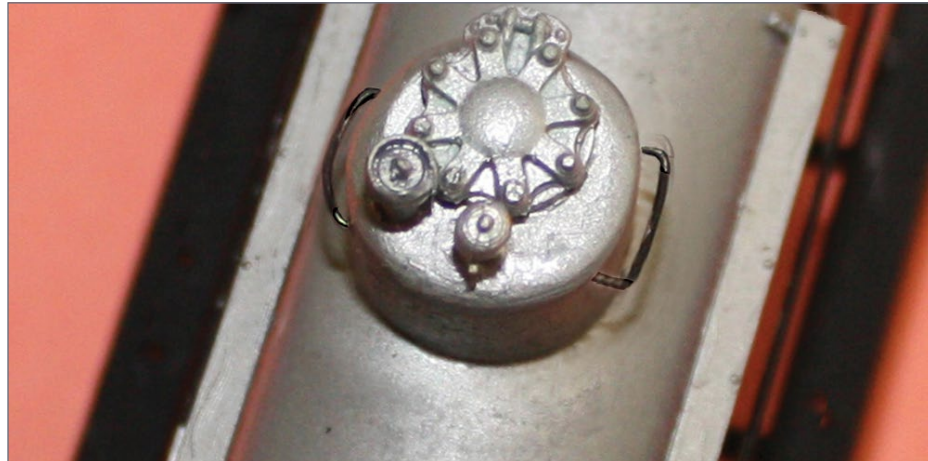
24. The dome top on the Becco peroxide car shown in [25]. As is typical, the manway cover is offset to one side, and a safety valve and access pipe cover are alongside it.
