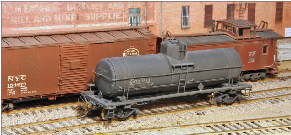
19. The completed 10,000-gallon tank car built by Richard Hendrickson from an Athearn tank car kit. Note that the tank bands at bolsters have been redone as separate bands. I inherited this model from Richard.
