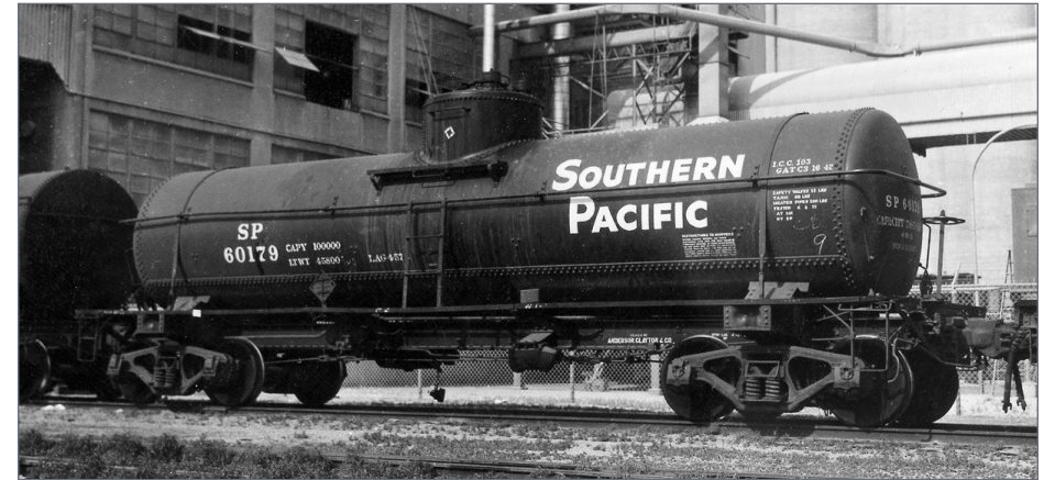
10. This SP tank car has a route card board (the pale rectangle above the running board, to the right of the ladder and above the brake cylinder), but the last clerk who attached a route card put it on the edge of the wood running board, above the left truck. The car, incidentally, is in cottonseed oil service and apparently empty; note the outlet pipe cap hanging from a chain under the car (this should have been closed). George Sisk photo at Kansas City, 1959, Charles Winters collection
