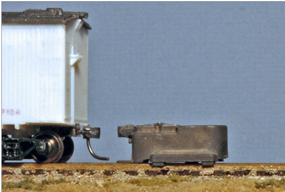
3. The Kadee gauge not only checks coupler height, but has a "shelf" below which checks height of the trip pin.
