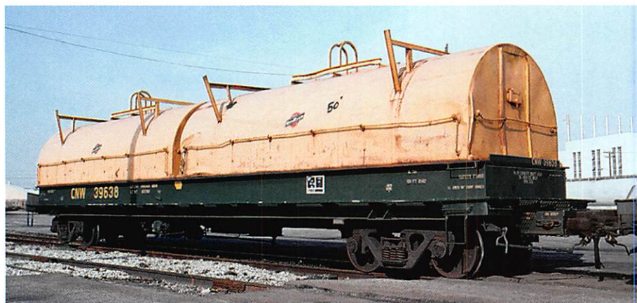
CNW 39638. Built by Thrall in September 1969. The car was painted by CNW's Clinton shops in February 1993. Interior length, 48' 11".
