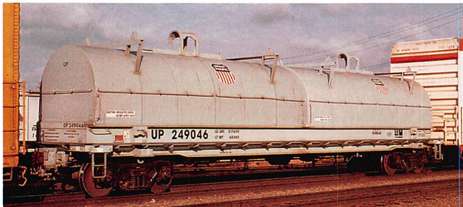
UP 249046. More or less the typical special-design purpose-built. Thrall built this one in December 1995. These have a pair of insulated hoods. Note the gray paint scheme, unusual for a UP car. March 1996; Omaha, NE.
