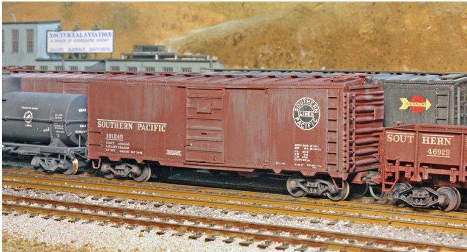
13. SP class B-50-27, modeled with a C&BT Shops kit cut down to 10 feet inside-height, with an added top end rib, upgraded detail parts, and Superior doors.
