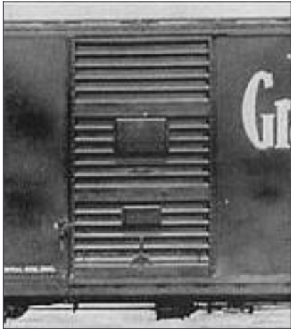
17. A Santa Fe car built in December 1945 by Mount Vernon Car Manufacturing Company has the interim version of the Youngstown door with wide horizontal join panels and centered door opener at the bottom.
