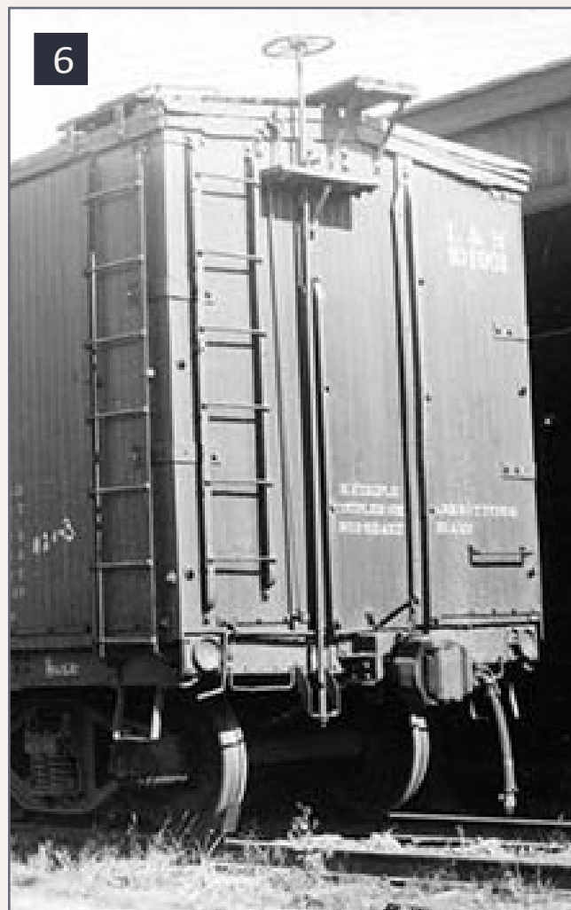
6. Double-sheathed wood car with unique vertical braces.
