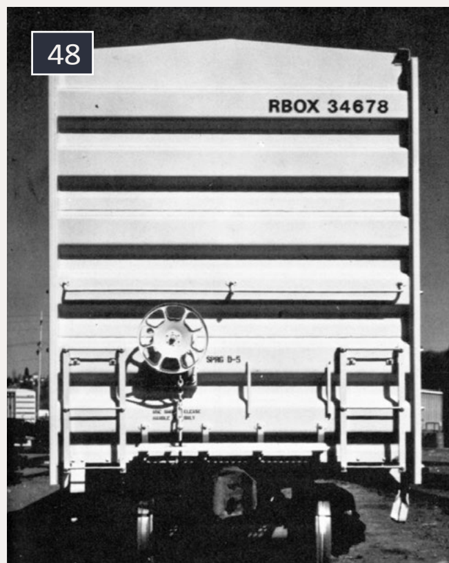
48. Pacific Car & Foundry built this RailBox car in 1979 using Stanray steel ends welded to the corner posts. The six non-terminating box corrugations are on 20" centers.
