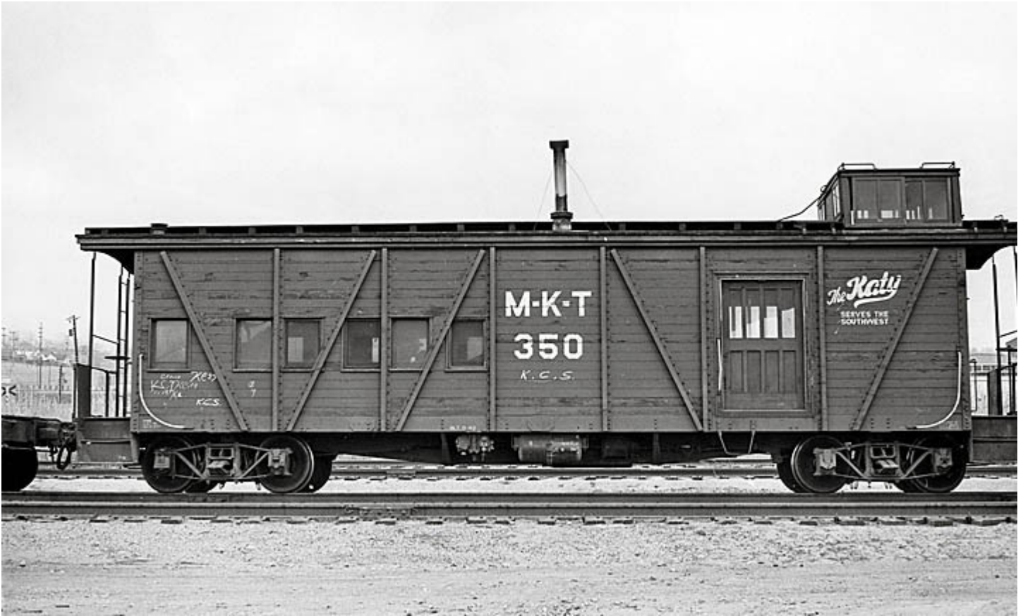
Missouri-Kansas-Texas drovers' caboose No. 350 shows off the car's extra length. The cars could accommodate extra riders overseeing livestock shipments. - Harold Schupp
