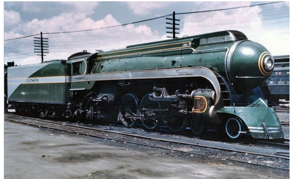
5. Streamlined Ps-4 Pacific #1380 was a rare example of streamlined steam on the normally conservative Southern railway. This locomotive retained its streamlining until it was scrapped in 1953. Photo by Heath Nicks
