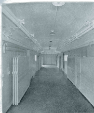
Car with Stall Equipment Stored, for Express or Baggage Shipments
